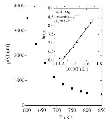
FIG. 3. Temperature variation of the resistivity ( $\rho$ ) of Mg-doped AlN in the temperature range of 600–850 K. The inset is the Arrhenius plot of  $\rho$ . The fitted value of the activation energy  $E_A$  is 0.50 eV assuming a temperature dependent hole mobility ( $\mu$ ),  $\mu \propto T^{-3/2}$ .
